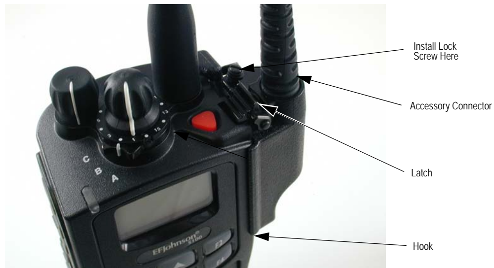
Figure 2.3 Accessory Installation
