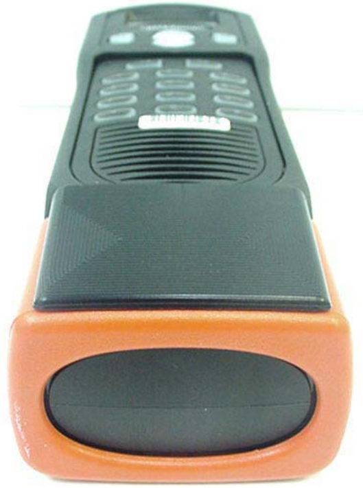
Bottom of DUT with Alkaline Battery Pack
