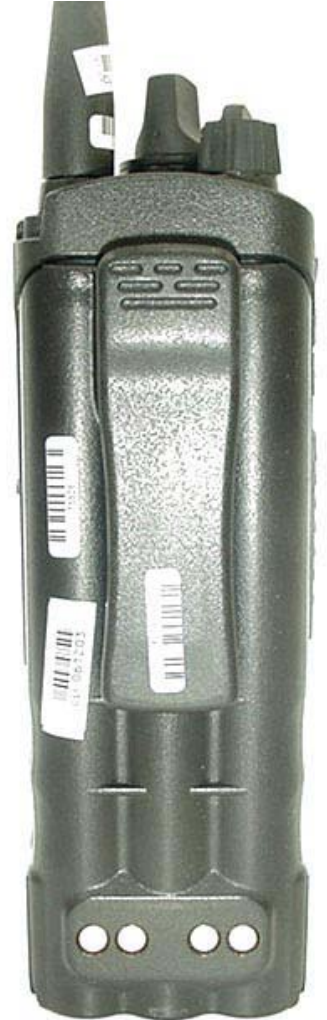
Back of DUT with NiMH Battery Pack with Belt-Clip
