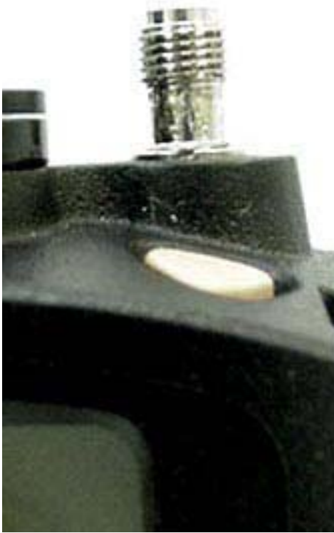
Radio RF Antenna Connector
