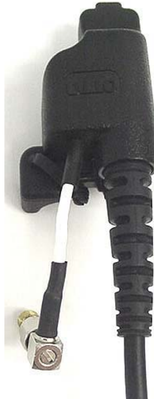
Speaker-Microphone-Antenna Connector & Terminator
