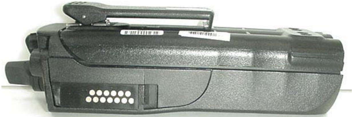
Right Side of DUT with NiMH Battery & Belt-Clip
