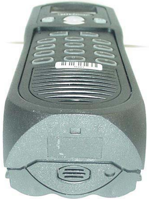
Bottom of DUT with NiMH Battery Pack
