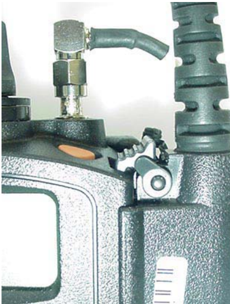
Front View of Antenna Termination
