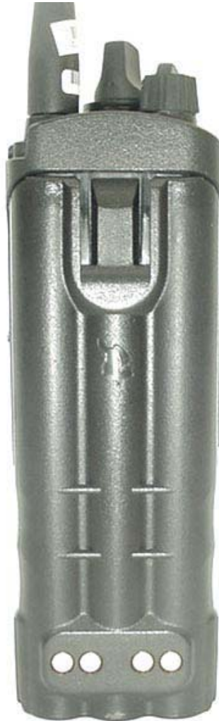
Back of DUT with NiMH Battery Pack
