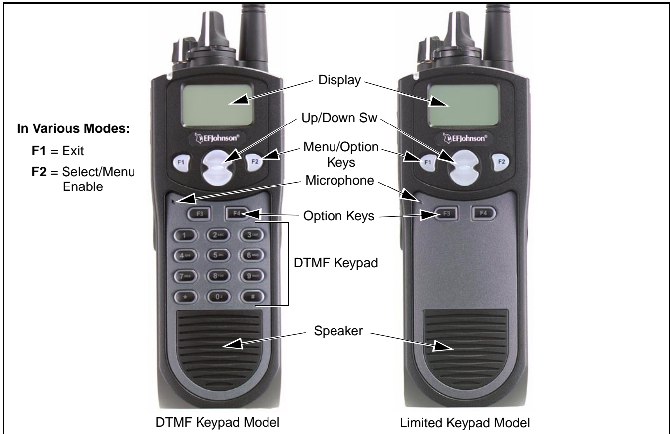
Figure 1 Front Panel Controls
